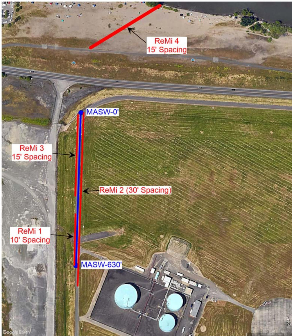
Figure 2-1. Site layout showing locations of geophysical arrays.
