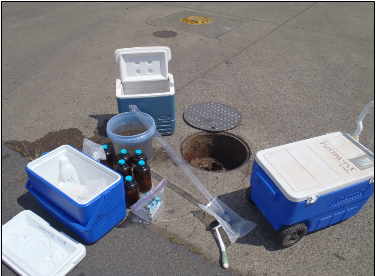
Photograph 2. Collection of the initial groundwater sample from the Observation Port. 5-6-2013.
