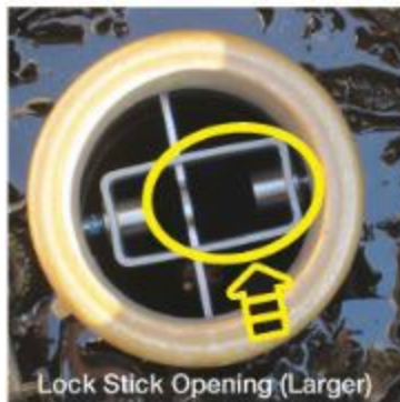
Lock Stick Opening (Larger) McGard Fuel Lock Installation Position 1
