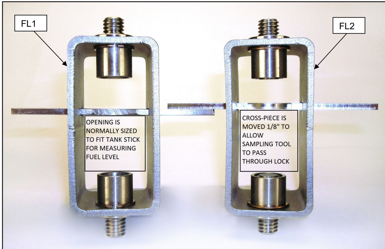
McGard Fuel Lock Installation Position 3
