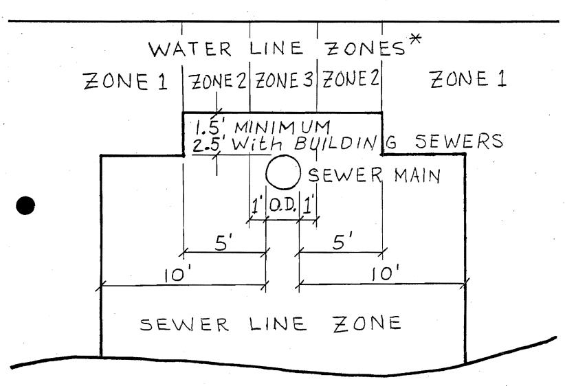
\* A PARALLEL WATER LINE SHOULD BE LOCATED ON UNDISTURBED EARTH IN ALL CASES,
