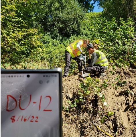
Sampling DU-12 0-1 foot interval – typical increment
