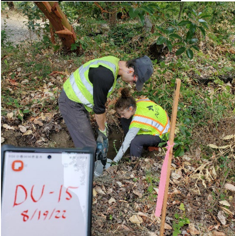
Sampling in DU-15 2-3 foot interval - typical
