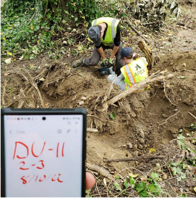
Sampling DU-11 2-3 foot interval – typical increment
