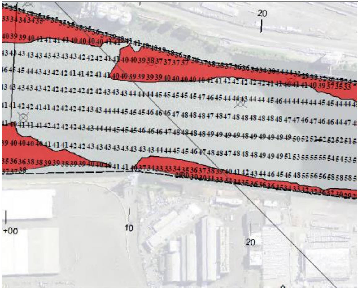
Figure 3. Bathymetry in the vicinity of Sulzer from 2014 USACE condition survey (USACE, 2014).
