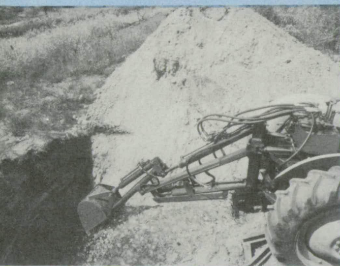
Digging irregular shaped hole from one position.
