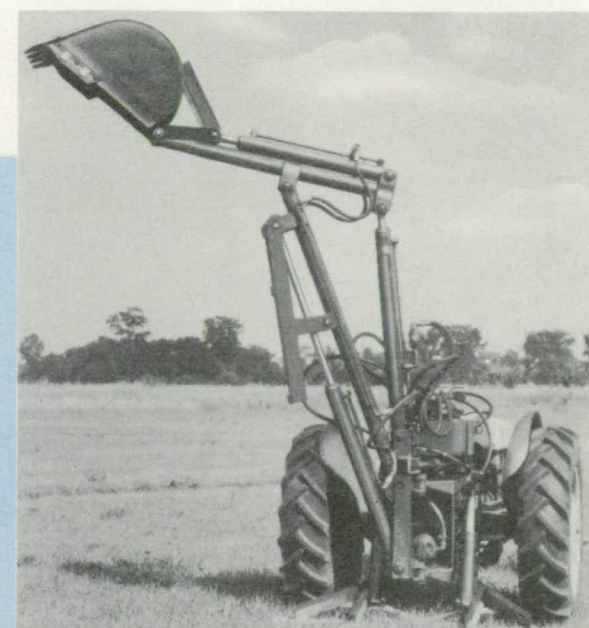
Shovel is hydraulically actuated
