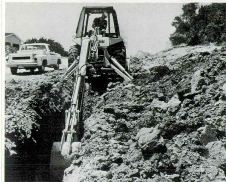
14'-18' telescoping Extendahoe provides up to 4' of extra reach and dig depth.
