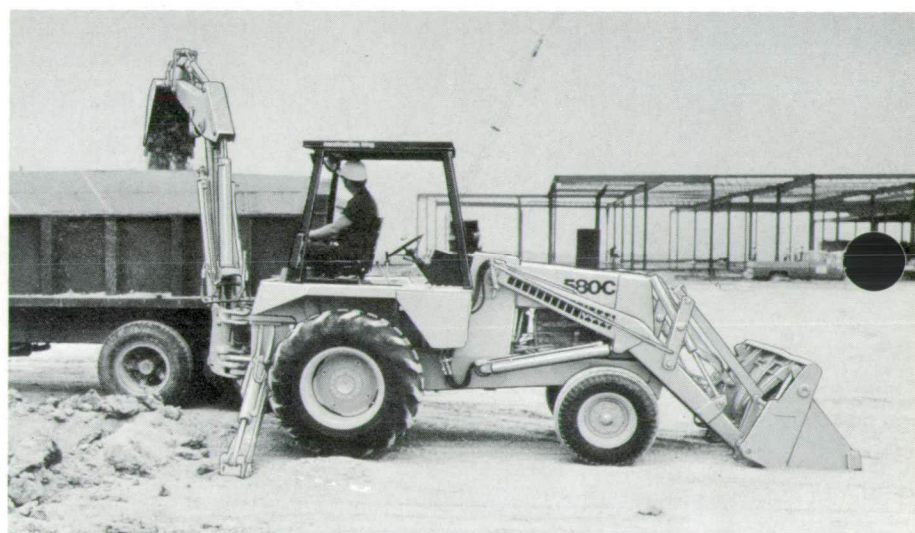
Standard 14' backhoe speeds excavating and truck loading cycles.
