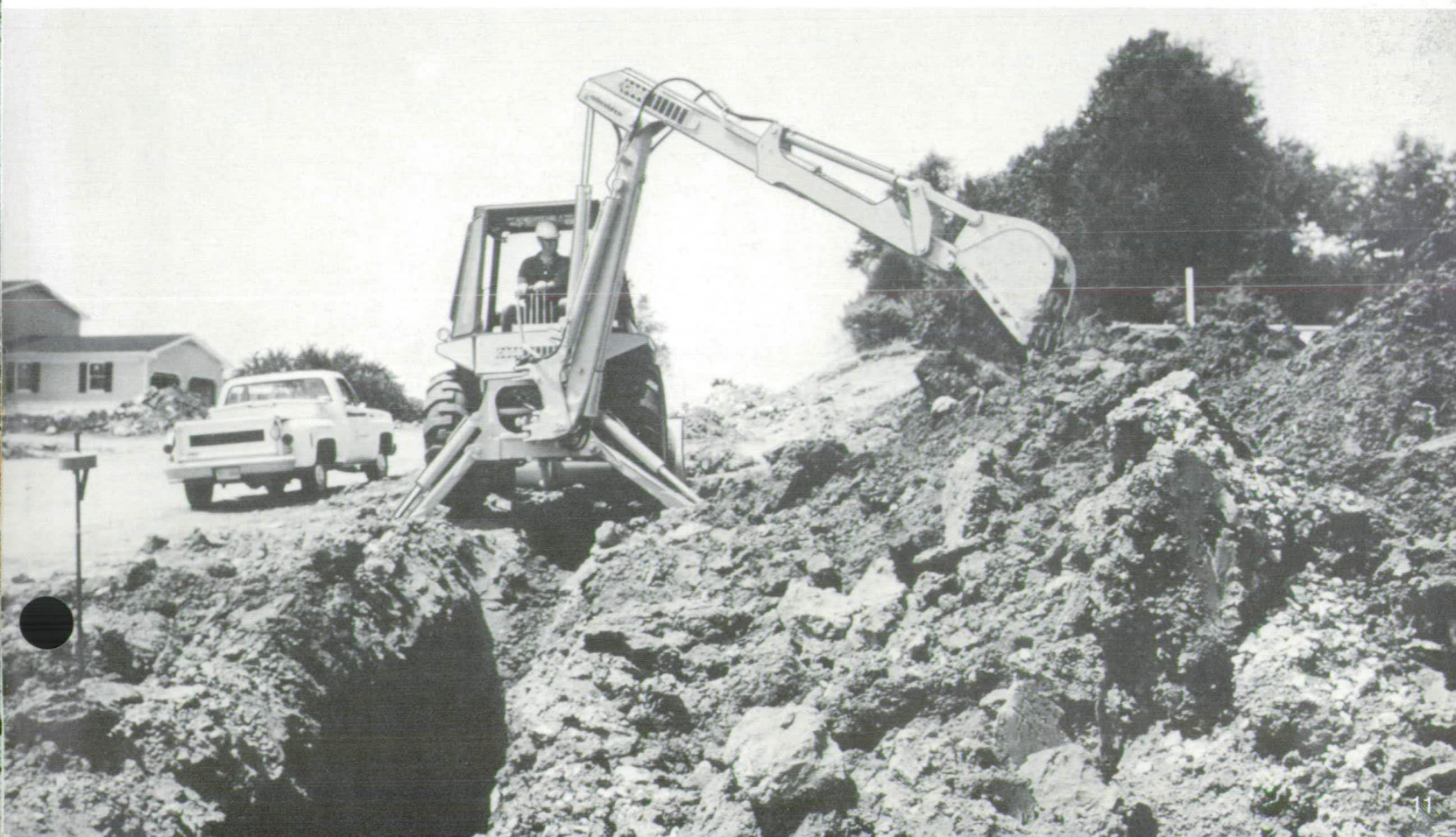
Hydraulic telescoping dipper permits digging of vertical holes.
