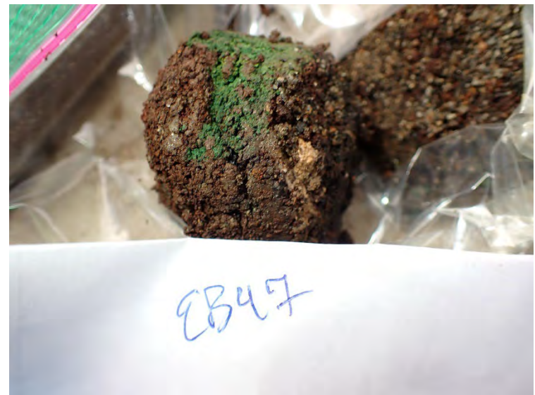
Apparent copper slag from EB47.
