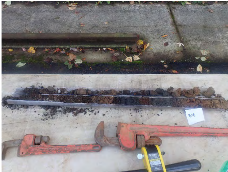
View of soil core from B08, revealing the gravel base rock beneath the asphalt surface.
