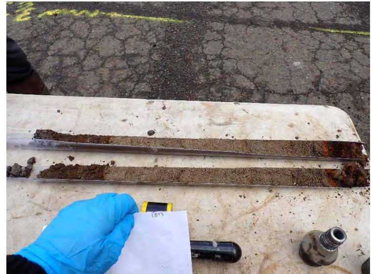
Medium sands encountered in EB43 inside the PIW building.
