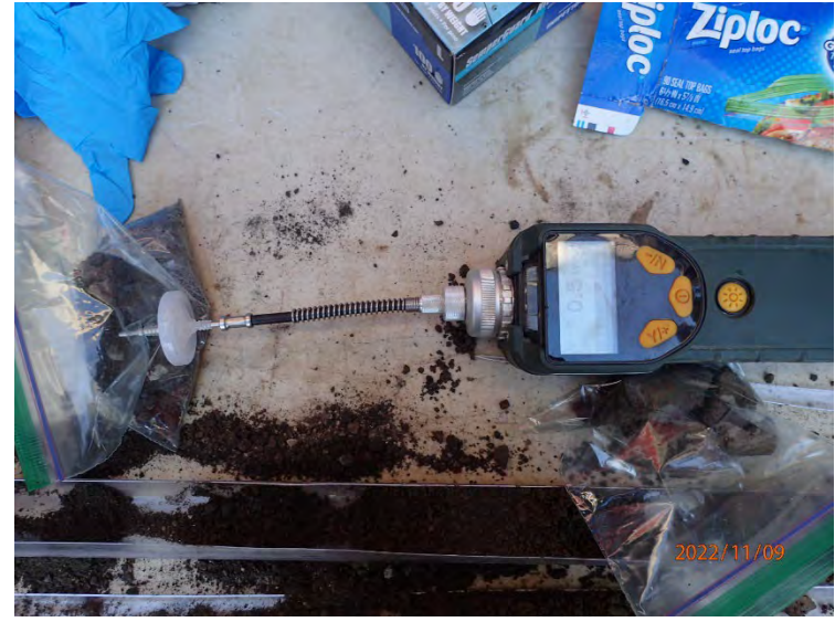
Using a PID to measure soil headspace measurements of a portion of the soil core.
