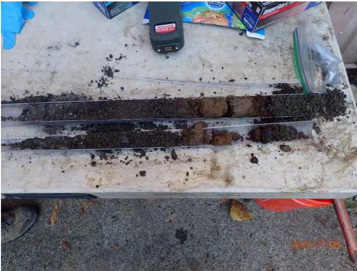
Soil cores were retrieved in plastic liners for field screening using a PID and collection of discrete soil samples.
