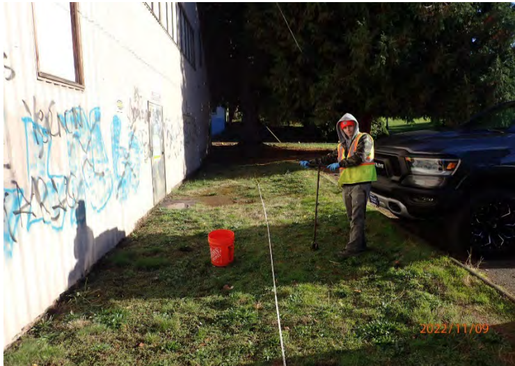
View east across decision unit DU01. ENW used a hand auger to collect and ISM sample and two replicate ISM samples from the area. A measuring tape was used to lay out the sample grid.
