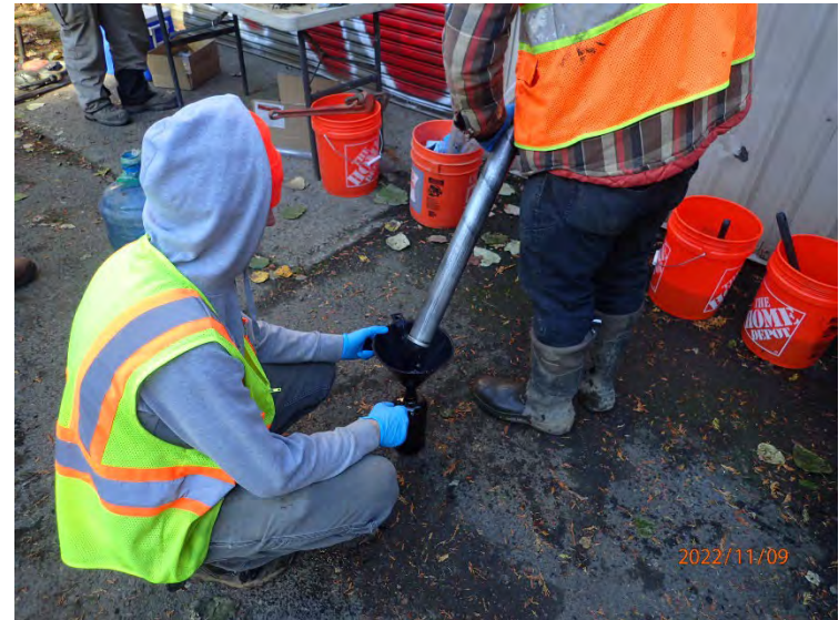
Equipment rinsate blanks were collected each day as part of the quality assurance/quality control program.
