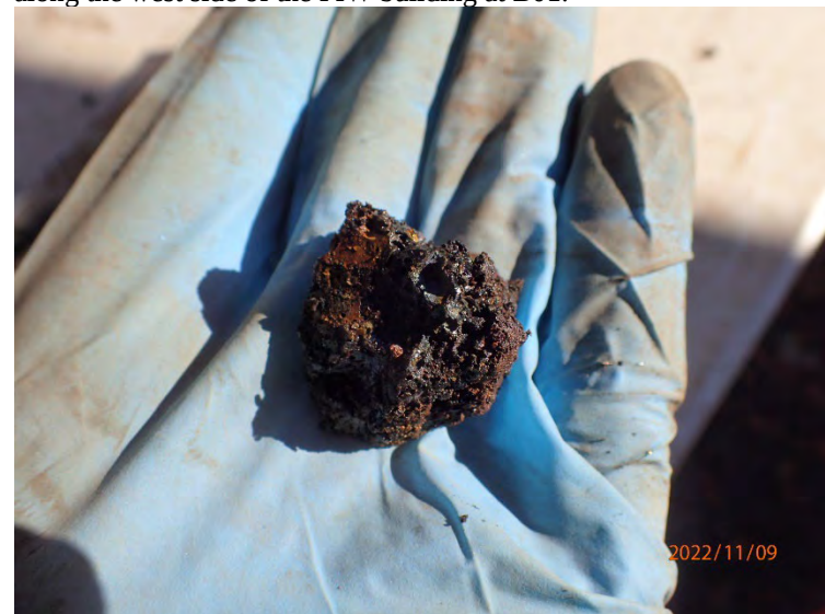
A piece of metallic slag found in the boring at B05.
