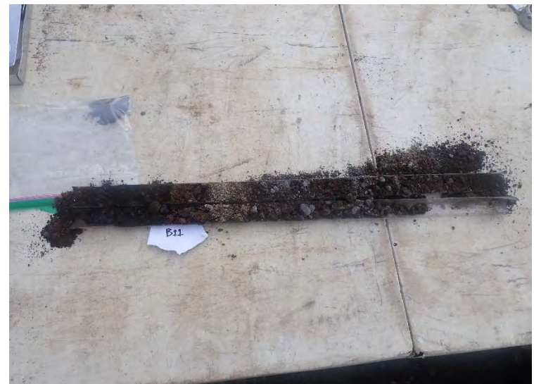
Soil materials recovered from B11, one of the borings with the highest PCBs detected in shallow soil.
