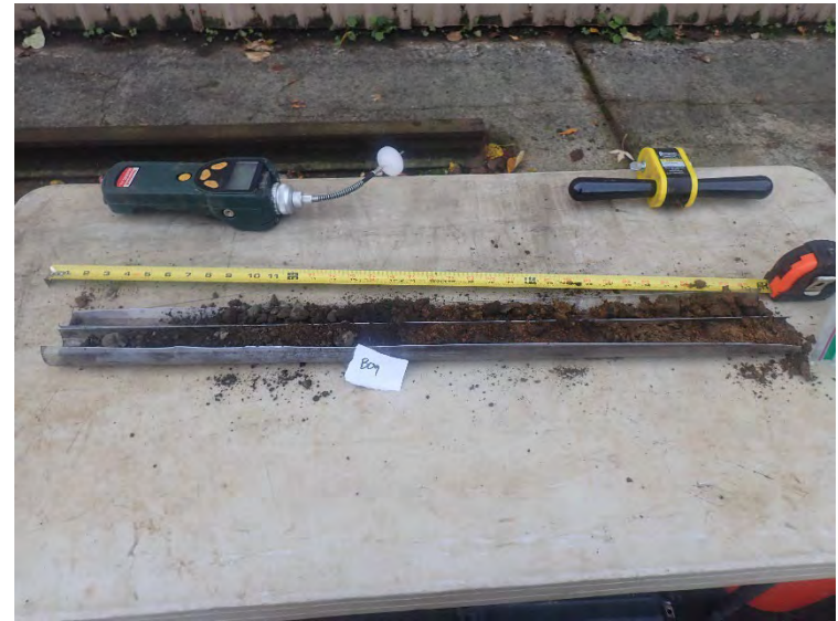
Soil materials encountered at B09 had the highest PCB concentrations of borings on the north side of the building.
