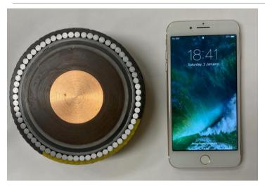
The main power cable is less than 6 inches in diameter; two cables are bundled with a fiber optic cable for burial in the riverbed.
