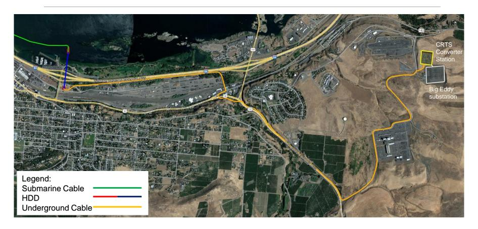
The Project Converter Station would be sited on approximately 6-acres adjacent to the existing Big Eddy substation. The underground cable would be buried along Columbia View Drive heading south to Route 197 (see next slide for additional route information).
