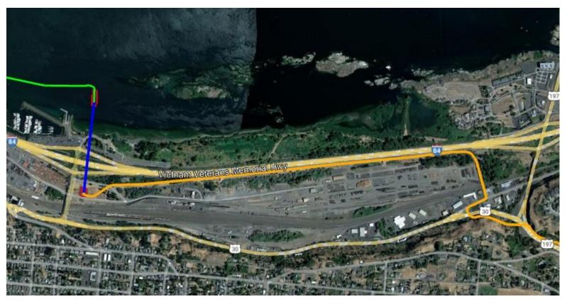
From Route 197, the cable would briefly run alongside Route 30 west and for a short distance on Second Avenue before crossing over a privately owned parcel to enter the Union Pacific Railroad complex. The cable would cross to the western end of the railroad property along Tie Plant Road. Using HDD technology, the cable would be routed underneath I-84 and property owned by the Port of Dalles and Wasco County Park to enter the River and proceed to the west.
