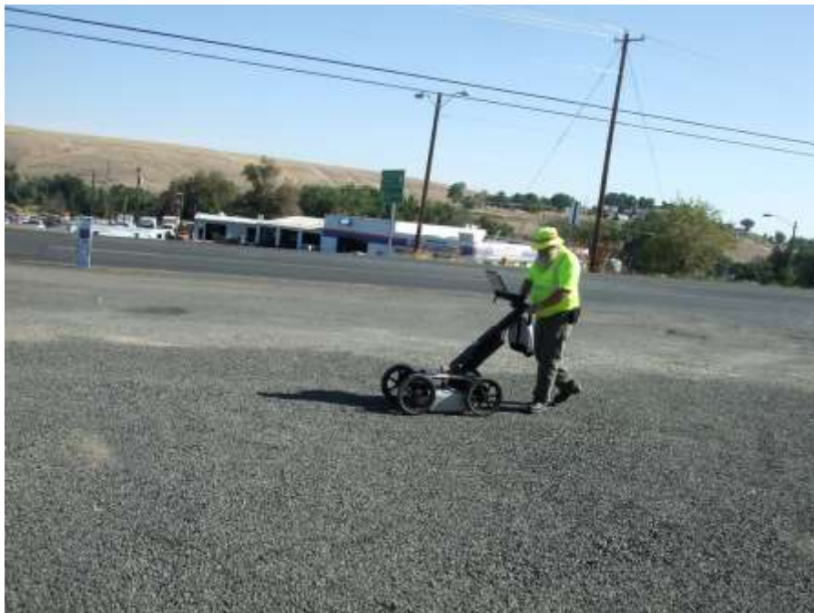
Photo 10. A view of the GPR survey.
