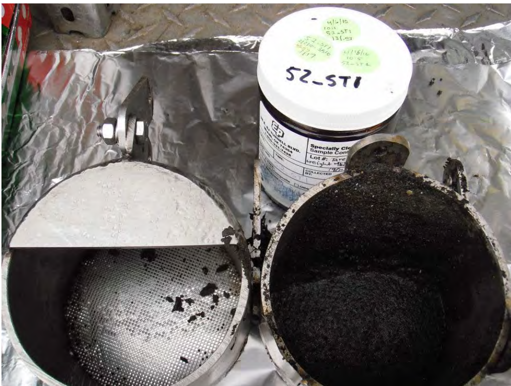
Photo 34 (June 16, 2010). Primary and secondary sediment trap chambers at time of removal.
