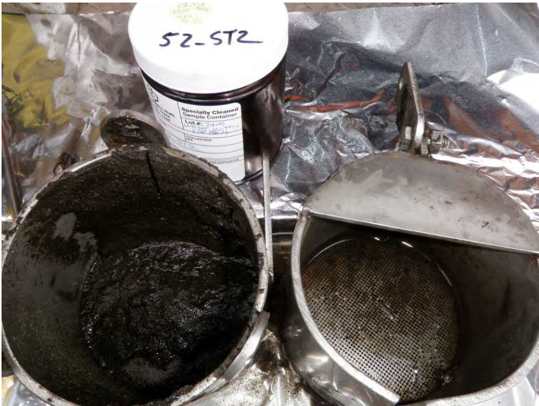
Photo 38 (April 6, 2010). Primary and secondary sediment trap chambers at monthly field check.
