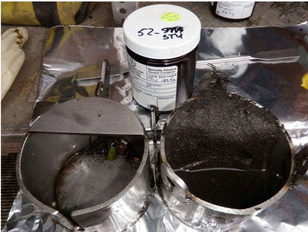
Photo 50 (April 6, 2010). Primary and secondary sediment trap chambers at monthly field check.
