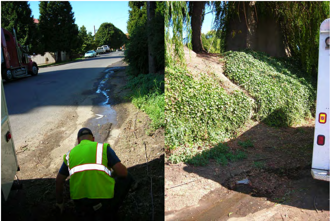
Photo 25a/b (September 9, 2008). Sampling location at catch basin AAE673. Water flowing into catch basin is wash water runoff from Independent Marine Propeller driveway (see Photos 21, 22).
