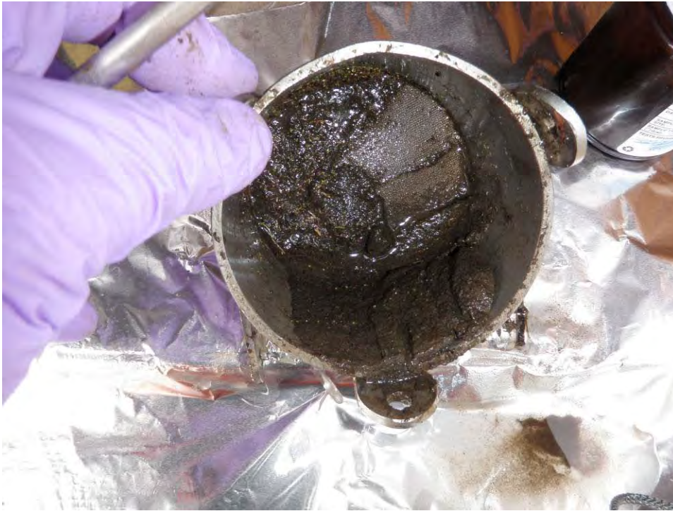
Photo 43 (April 6, 2010). Secondary chamber of SIFT© sediment trap, with solids present at time of monthly field check.
