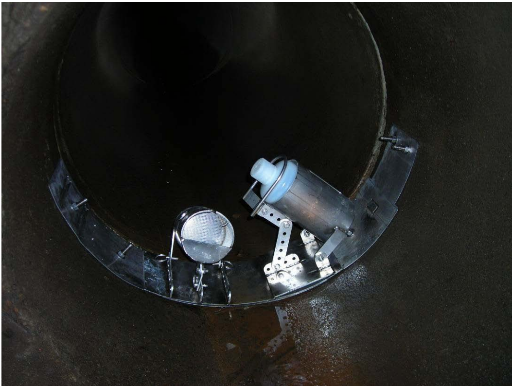
Photo 42 (February 2, 2010). SIFT© and standard sediment trap installed side by side in the 28-inch line exiting manhole AAE700).
