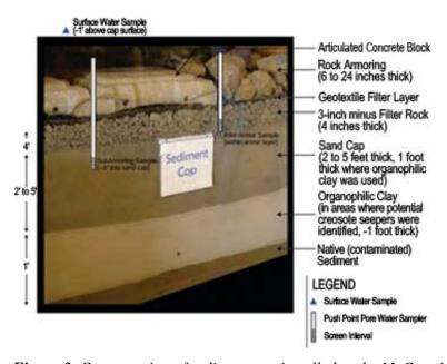
Figure 3. Cross-section of sediment cap installed at the McCormick & Baxter site.
