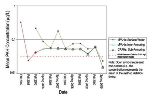
**Figure 6.** Mean concentrations for total cPAH in surface water, inter-armor water (collected within the rock armor), and sub-armor (sand cap) water of the sediment cap at the McCormick & Baxter site.
