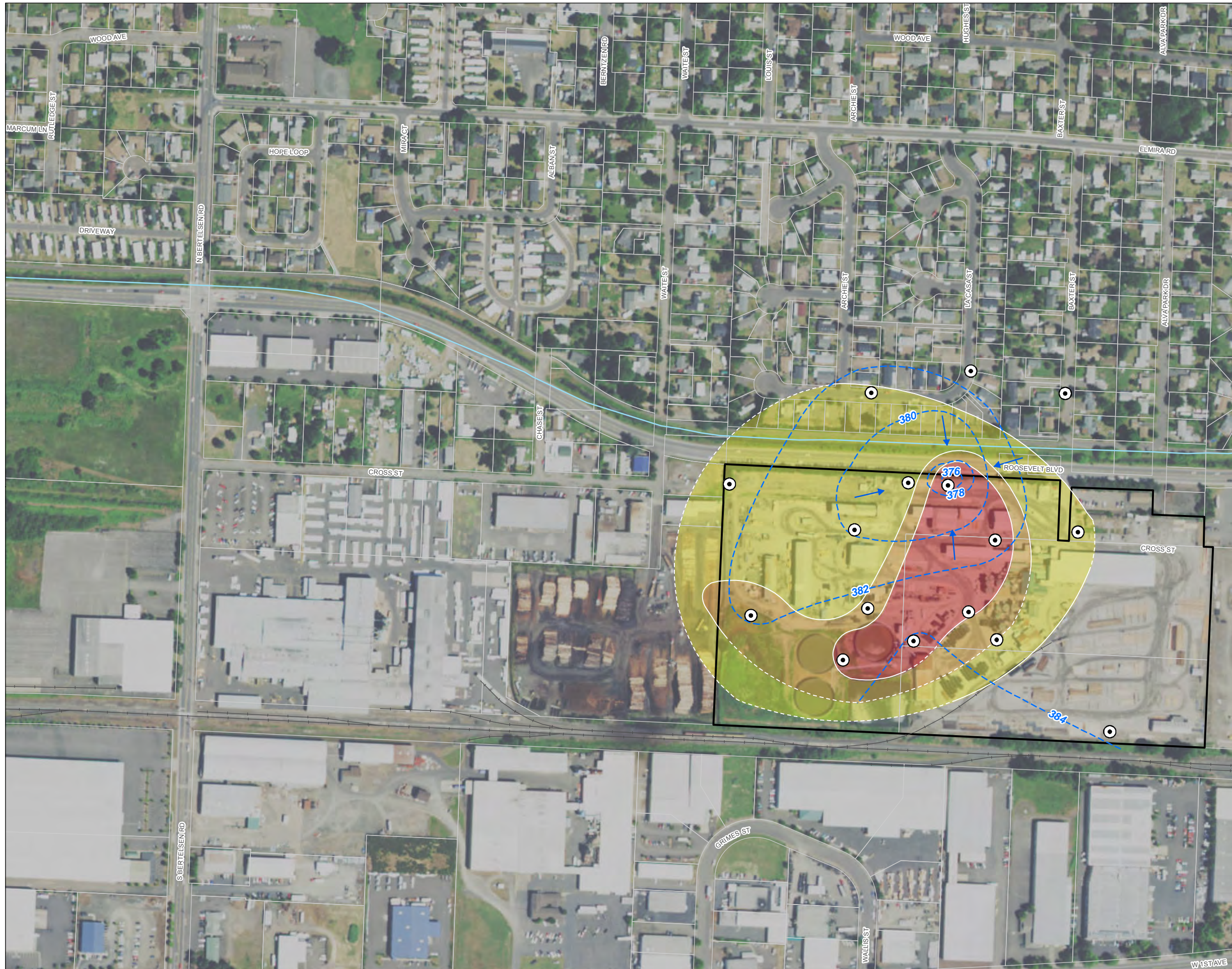
FIGURE 10-4 PCP Concentrations in Shallow Monitoring Wells 2001 or Maximum Concentration Prior to 2001 JH Baxter Eugene, Oregon
