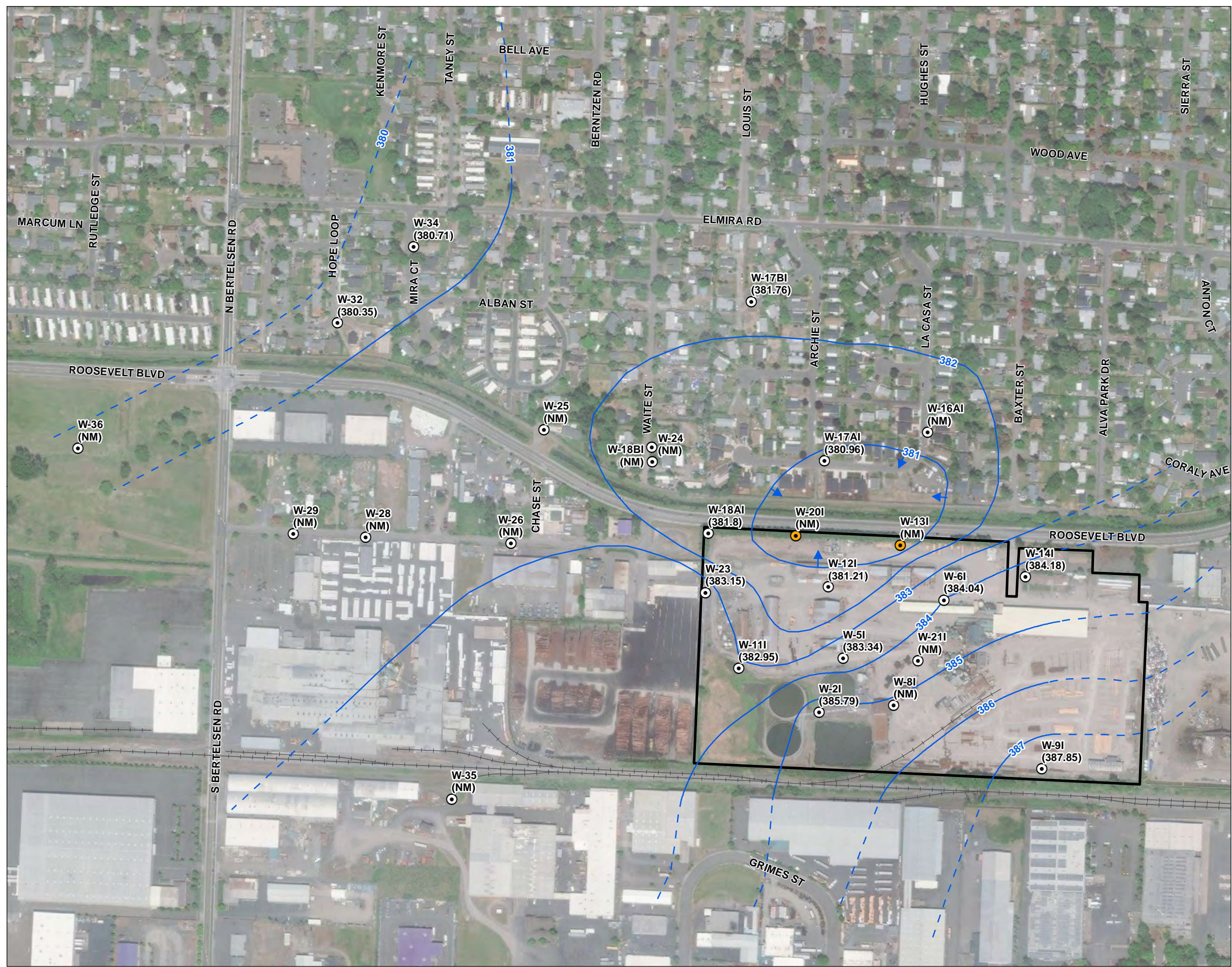
FIGURE 4 Intermediate Zone Groundwater Elevation, First Half 2020 J.H. Baxter Wood Treating Facility Eugene, Oregon
