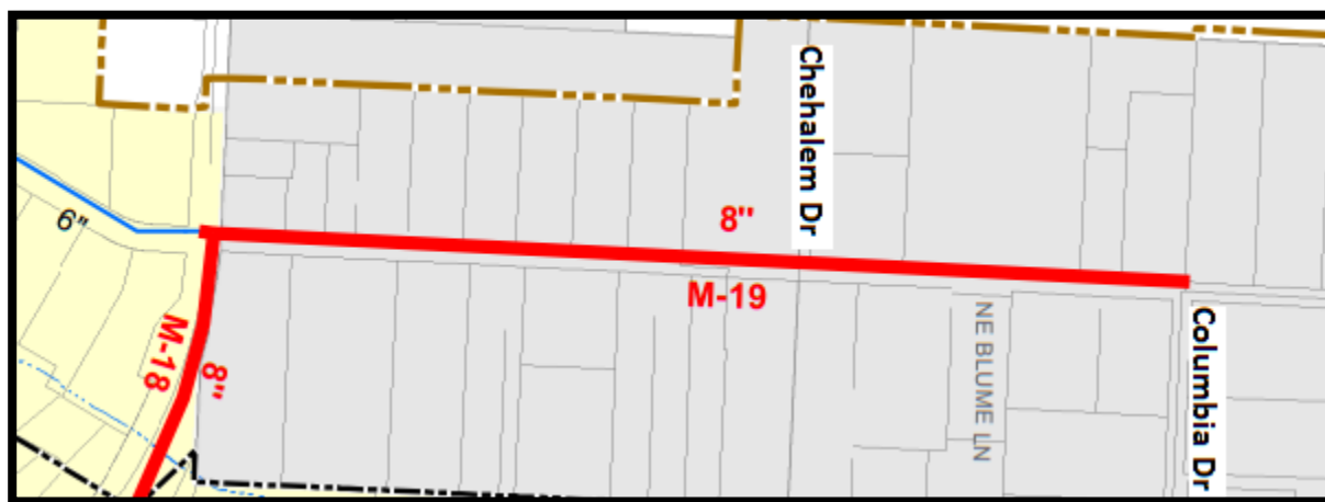
FIGURE 4 CHEHALEM DRIVE PUBLIC WATER SERVICE LINE EXTENSION
