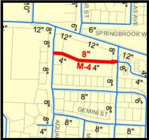
FIGURE 44 EXPANDING WATERLINE TO ELIMINATE DEFICIENT WATER FLOW AND FOR FUTURE GROWTH
