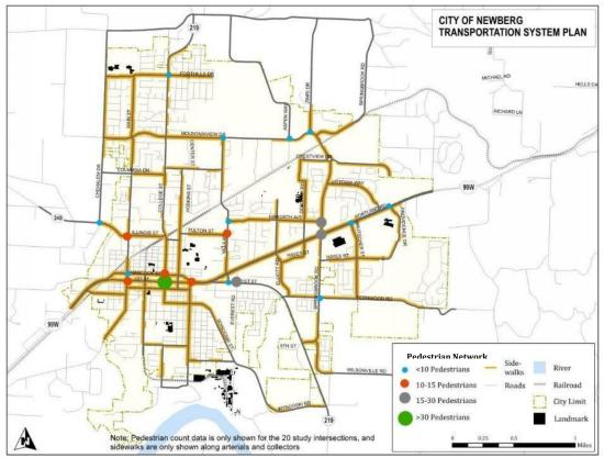
Figure 3: Pedestrian Volumes and Existing Sidewalk Network
