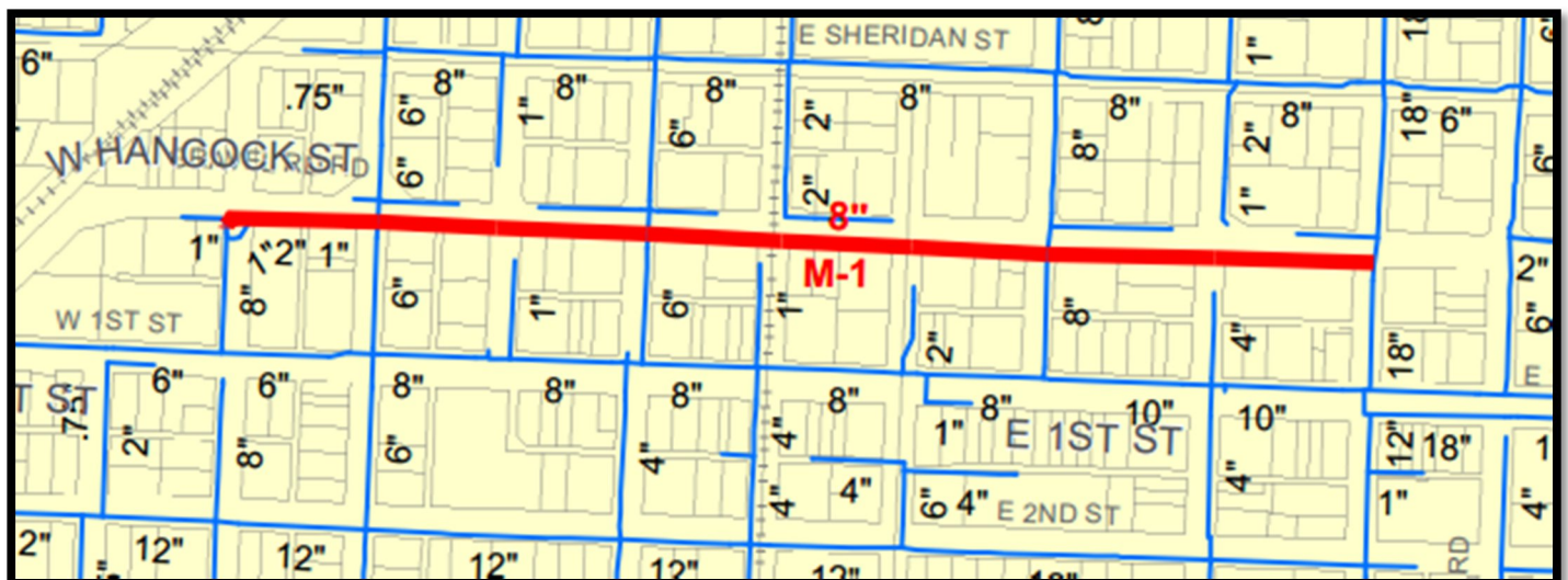
FIGURE 22 REPLACING DEFICIENT PIPE AND INADEQUATE FIRE HYDRANTS ON HANCOCK STREET
