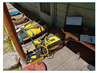
and Strong Gradient arrays with electrode spacing of 3 m along four lines composed of 21 electrodes each. Depth of exploration was on the order of 40 feet below grade.
