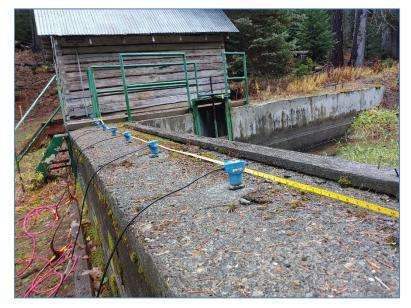
of the dam's character. However, at a depth of roughly 12 feet below the top of the dam, the model suggests a velocity reversal to lower strength material. This reversal is well constrained by the data and, in the opinion of SA, represents the transition from the concrete structure to native foundation soils probably composed of granular, unconsolidated materials.
