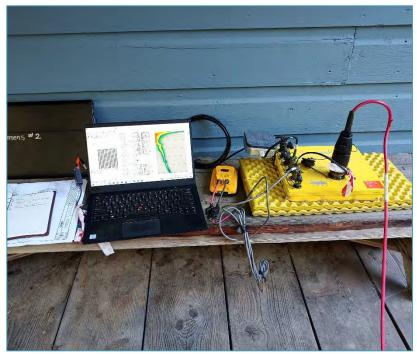
the first arrival wave at the receiver is considered in the SR method. These first arrivals are picked for each shot at each receiver. As the energy travels through the ground, the waves are refracted and the arrival time, combined with distance from the source, is related to both the velocity and distance to the layers promoting refraction. This distance is not necessarily vertical depth; rather the nearest refractor and the image can be skewed when oriented along a dipping refractor.
