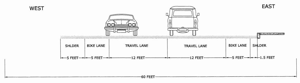
WEST 10TH STREET ROAD RIGHT-OF-WAY = 60 FEET CURRENT CROSS SECTION @ CHENOWITH LOOP
