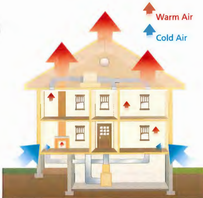
Fig. 10. The pattern of air movement referred to as the "stack effect". Illustration: Blank Space LLC.
