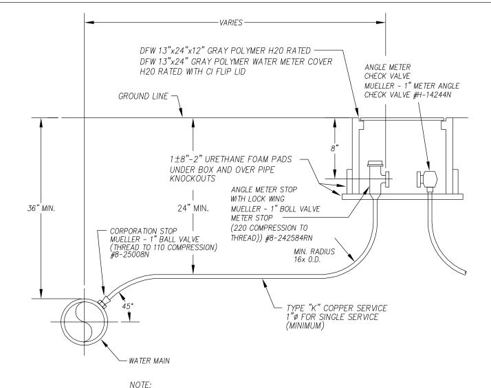
NOTE: DIRECT TAP MAY BE MADE TO ALL SIZES OF DUCTILE IRON MAIN FOR 1" SERVICES. ALL OTHER SERVICE CONNECTIONS SHALL BE MADE USING A SERVICE SADDLE AT THE MAIN. TRAFFIC RATED METER BOX AND COVER REQUIRED IN AREAS SUBJECT TO VEHICLE TRAFFIC.
