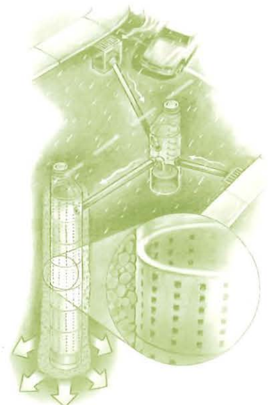
Sumps collect stormwater allowing runoff to soak into the ground.
