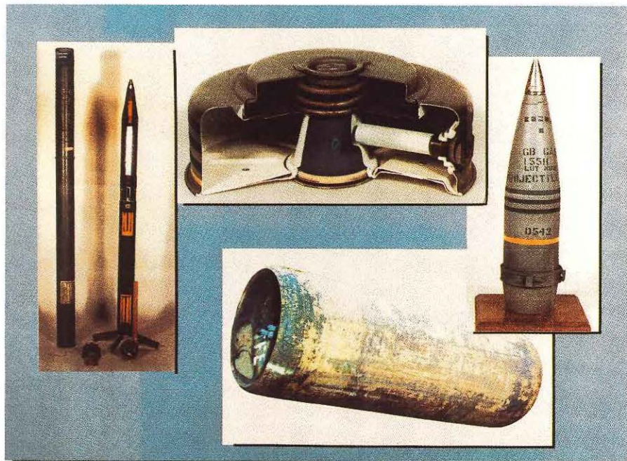
Chemical agents have been placed in projectiles, mines, rockets, and stored in ton containers.
