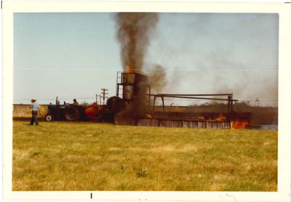
Sanitizer #75-03 operating in 1975 in a bluegrass field with considerable regrowth and heavy thatch, resulting in excessive black smoke emissions. The black smoke is characteristic of bluegrass only but is not excessive in a "normal" year.
