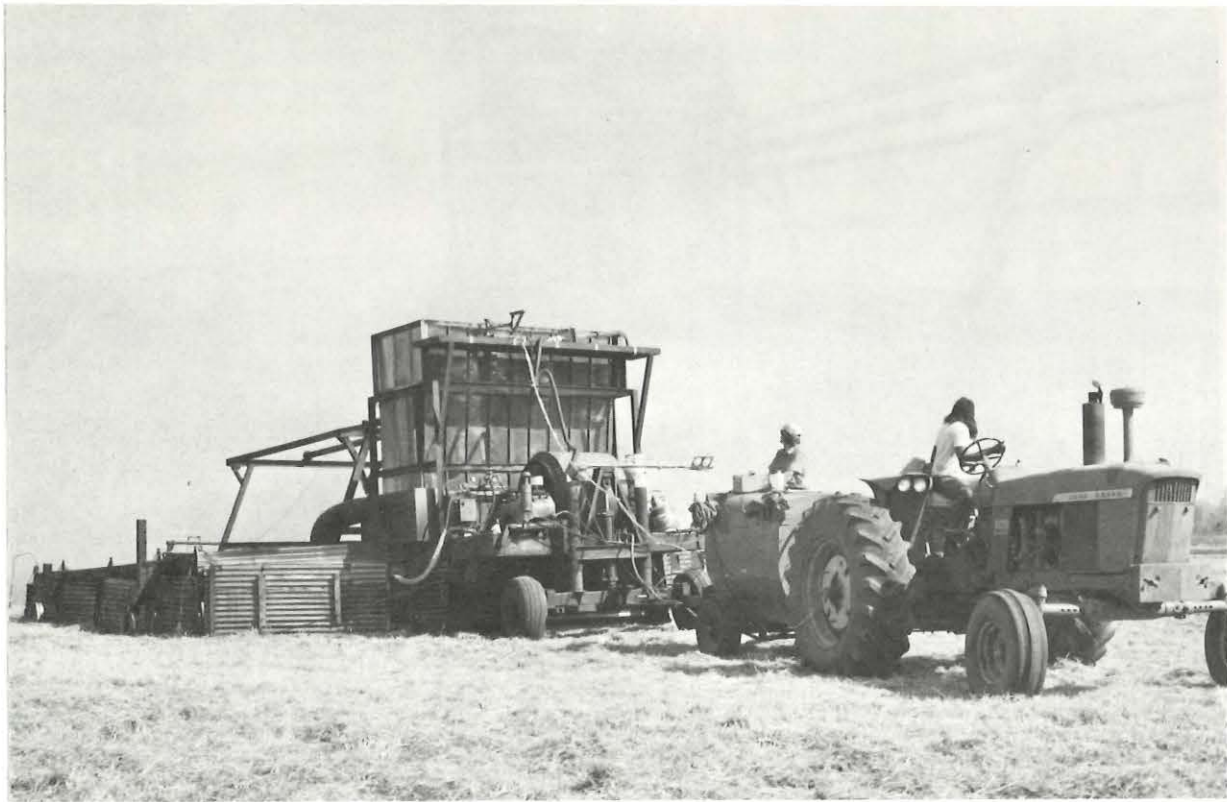
Sanitizer #75-02 (24' wide), with multi-air-bar deck being stack-emission tested on perennial ryegrass field in 1976.
