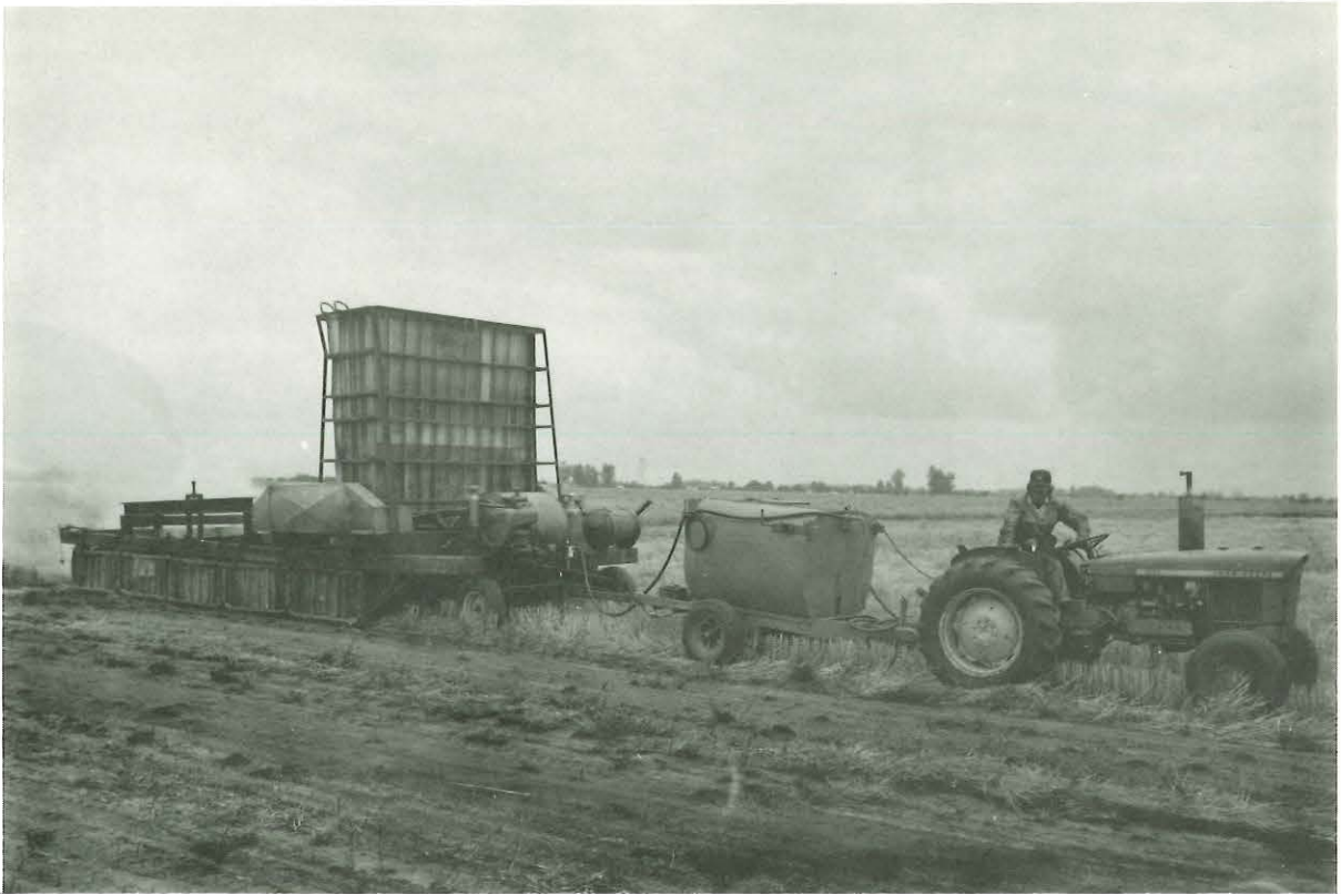
Experimental Prototype #75-04 (10' wide) with revised deck test burning a 5.3 Tons/Acre wheat stubble field in 1976.
