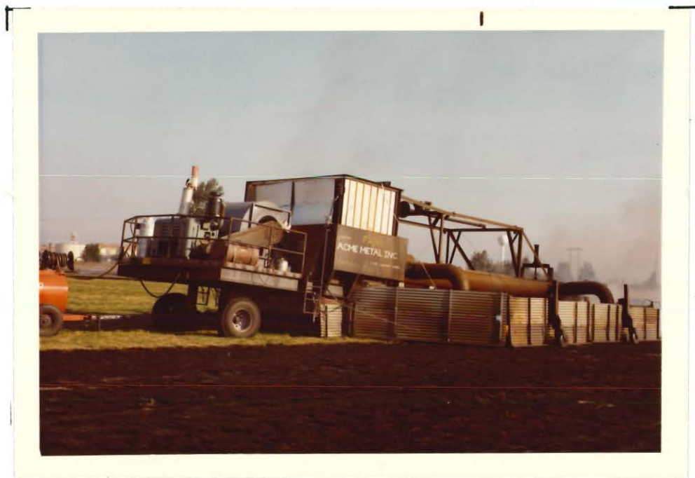
Sanitizer #76-05 on a well-prepared bentgrass field with regrowth caused by rain and delayed harvest and straw removal. Note uniform sanitizing in foreground.
