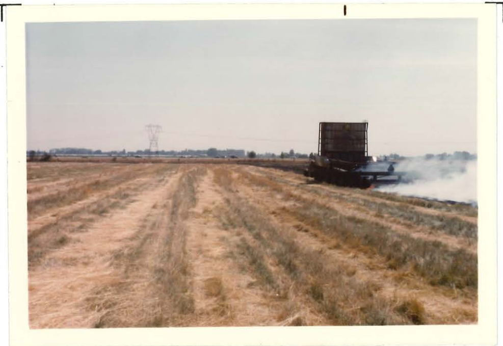
Sanitizer #75-04 test burning a fescue field in 1976 with very poor straw removal. Note windrows of straw which create alternate hot strips on field, and reduce capacity.
