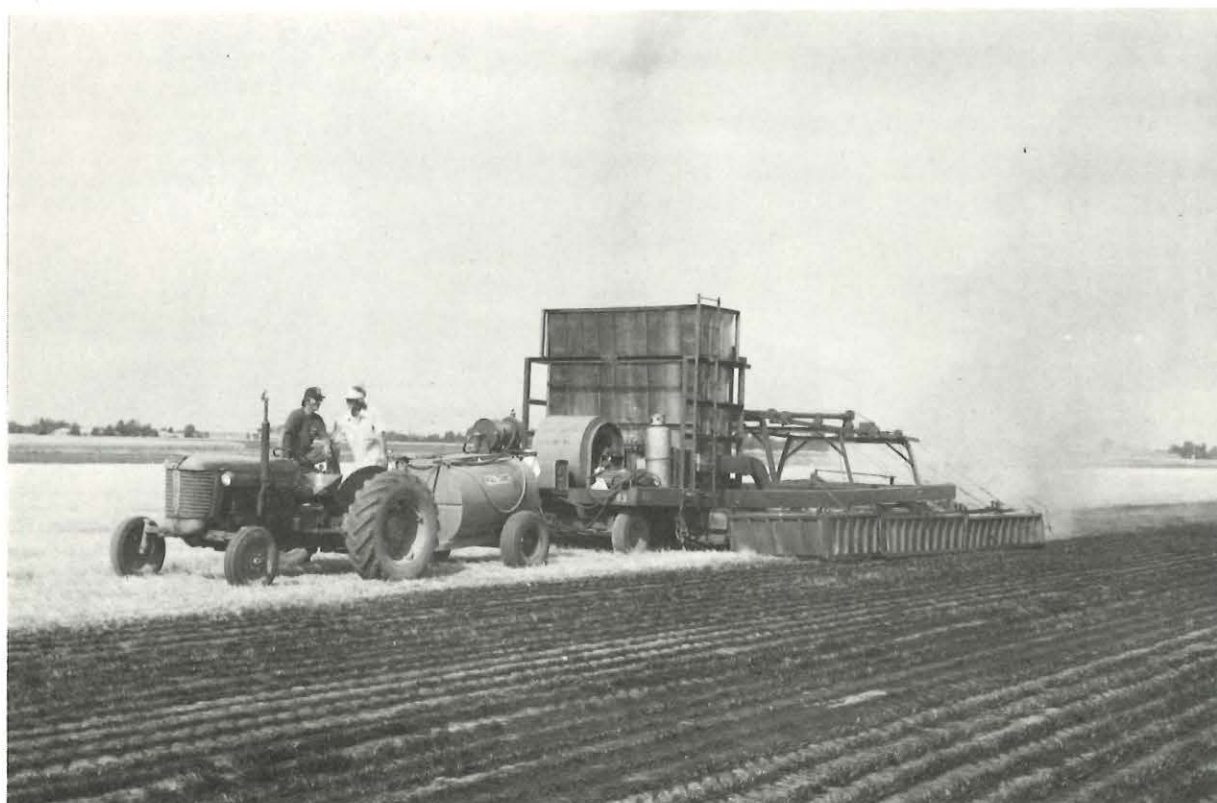
Sanitizer #75-03 (22' wide) with new s/s skins sanitizing a very well-prepared fine leaf perennial ryegrass field, averaging 4A/Hr for 36 Acres, in 1976.
