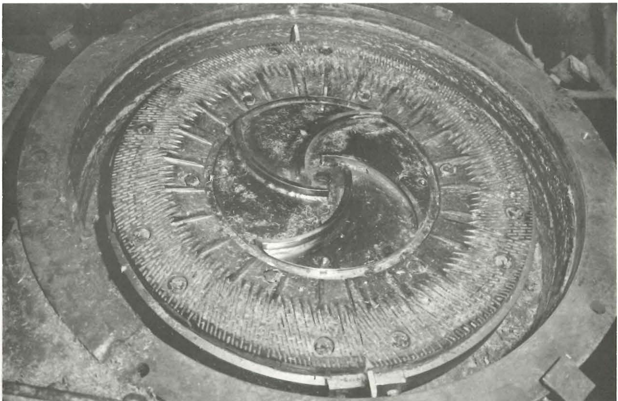
The rotating 28" disc of the Jones Vertifiner being used to defiberize straw. A matching stationary plate with center feed opening is mounted with .005" to .0010" clearance.
