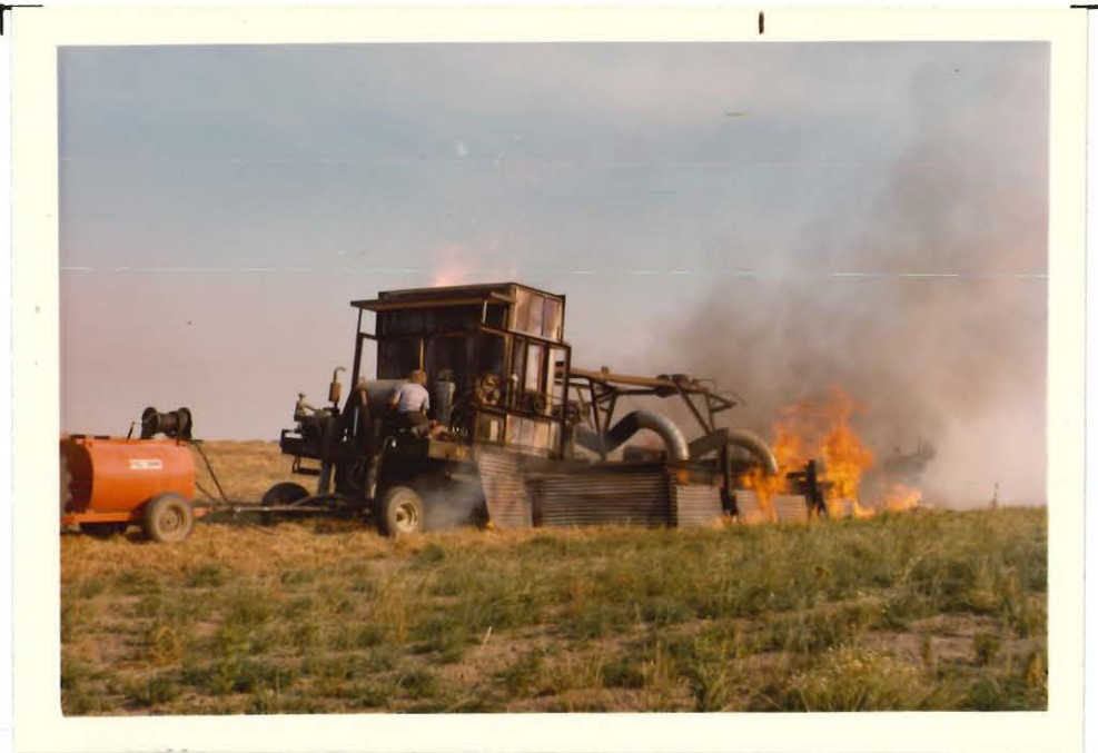
Sanitizer #75-01, with new plenums for 1976, briefly test-burning a very dry field of orchardgrass with all the straw left on (5.1 T/A). The excessive fuel (equiv. 500 g oil/A) would have damaged both machine and crop if continued.
