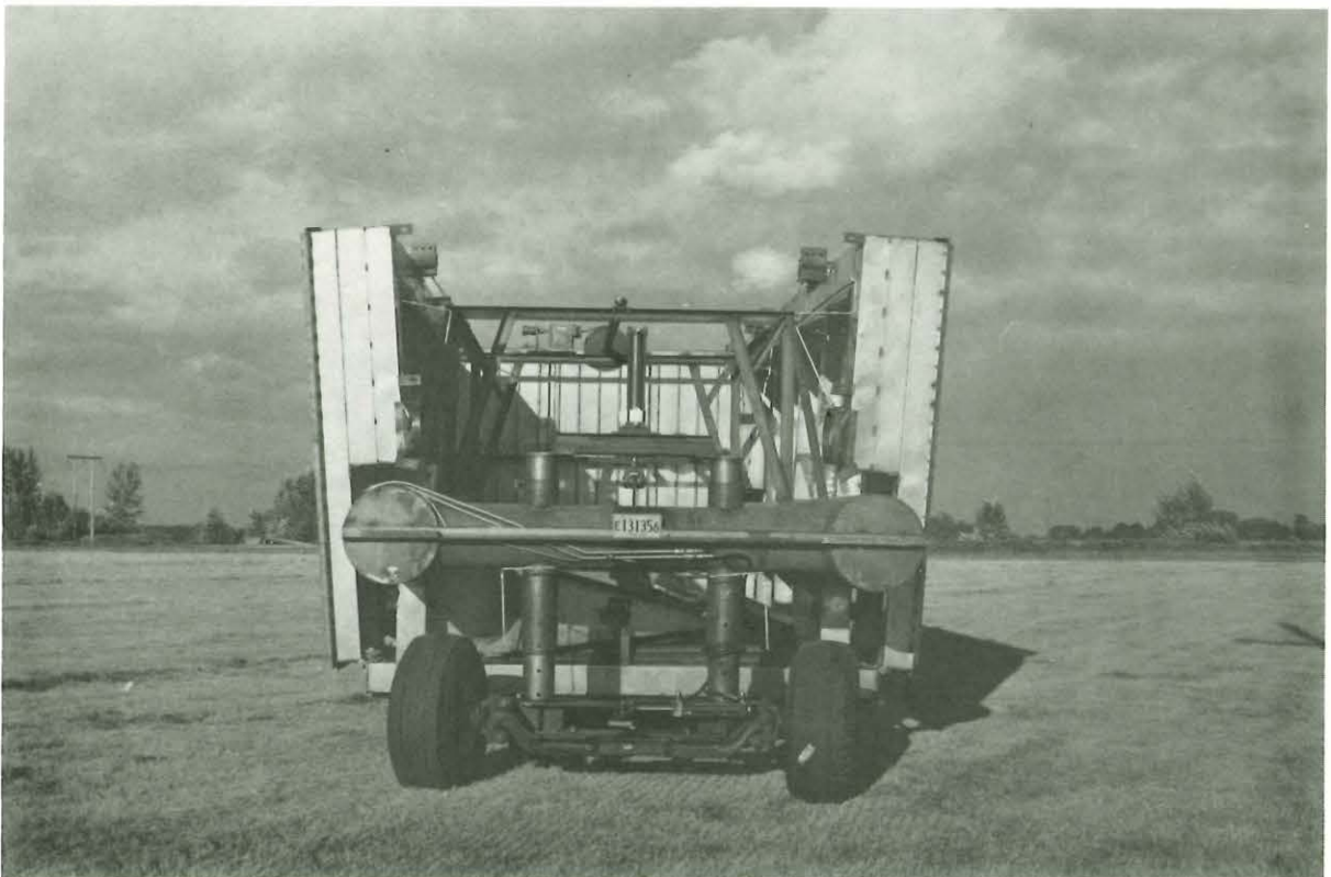
The 10' wide wings on #76-05 being lowered to provide a 32' burning width. Water-cooled steel wheels replace the rear tires used for road travel.
