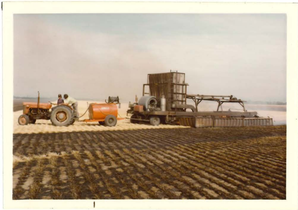
Sanitizer #75-03, with new stainless steel skins for 1976, operating in a well-prepared fine leaf perennial ryegrass field.
