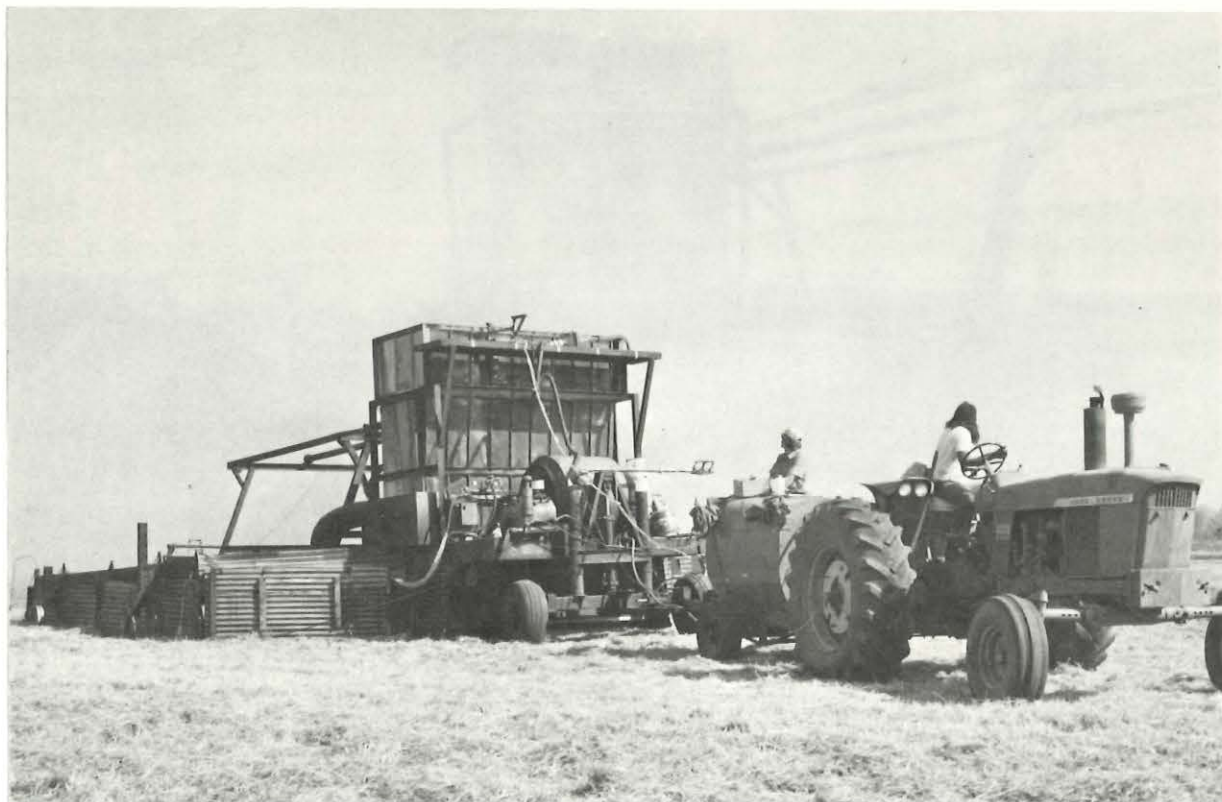
Sanitizer #75-02 (24' wide), with multi-air-bar deck being stack-emission tested on perennial ryegrass field in 1976.
