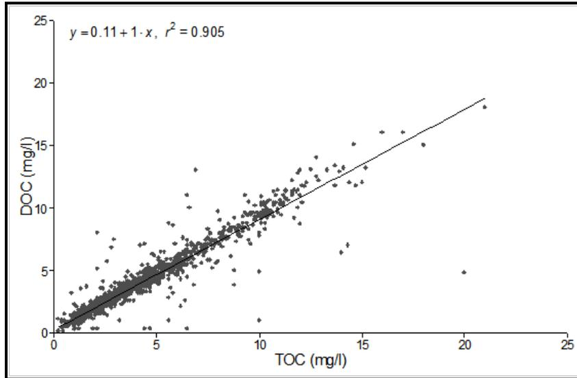
Using a translator of 0.83 was relatively accurate for predicting measured DOC values from paired TOC data (**Figure 10**). The root mean square error was 0.99 mg/L DOC, about equal to the DL of DOC for most samples.
