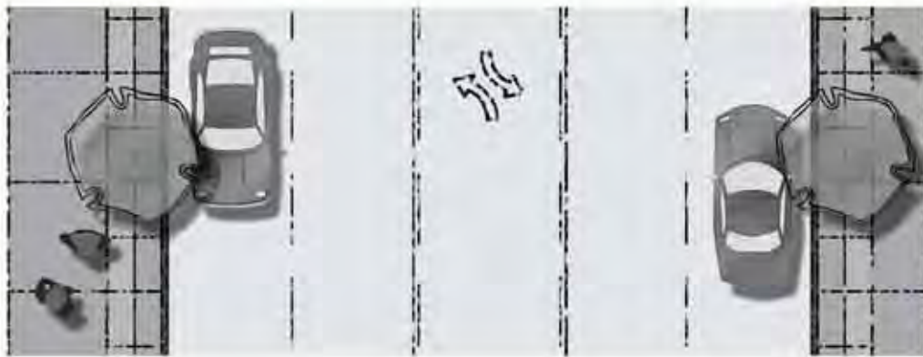
Figure 5: Furnishing Zone with Street Trees. If the sidewalk corridors were increased to the 12-foot standard or greater through acquiring additional right-of-way, the Through Pedestrian Zone and Furnishings Zone would be functionally wide enough to accommodate streets within the Furnishing Zone behind the curb lines. This is typical of urban commercial streets and provides a pedestrian buffer and visual attractiveness. This would likely require a Design Exception for the trees.
