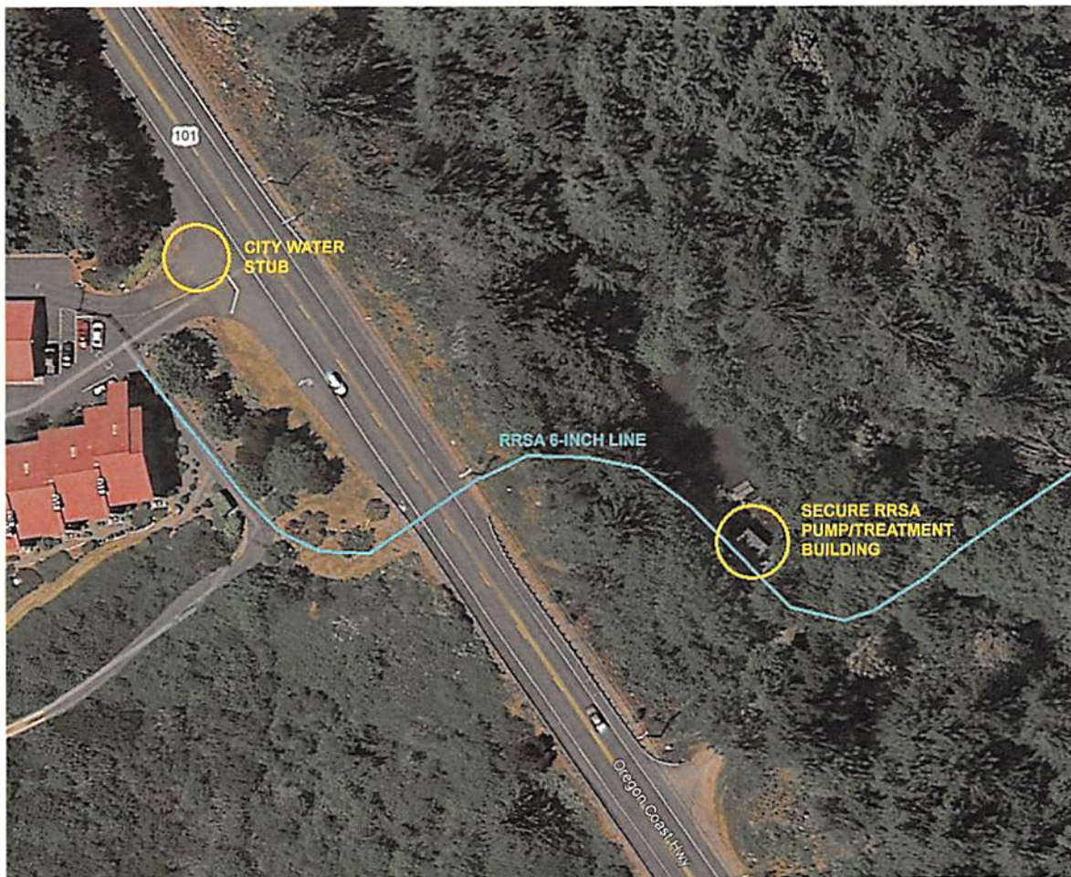
Figure 4 - Location of the City stub for the RRSA system connection to City water.
