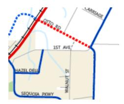
The earlier drafts of the TSP update (including the May 2010 draft) showed the intersection of Walnut Street and SE 1<sup>st</sup> Ave being constructed as a roundabout when the connection to Otto Rd and OR 99E is established. The latest draft shows the intersection's traffic control as a 4-way stop rather than a roundabout (Figure 7-9 (page 7-32)).
