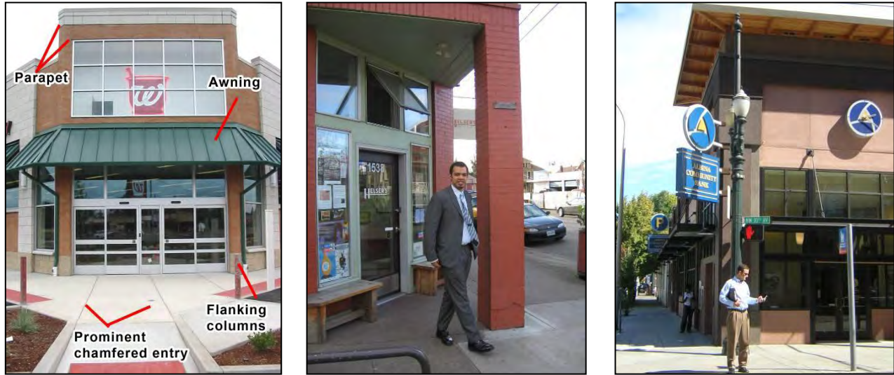
Figure 63 Corner of building elements
