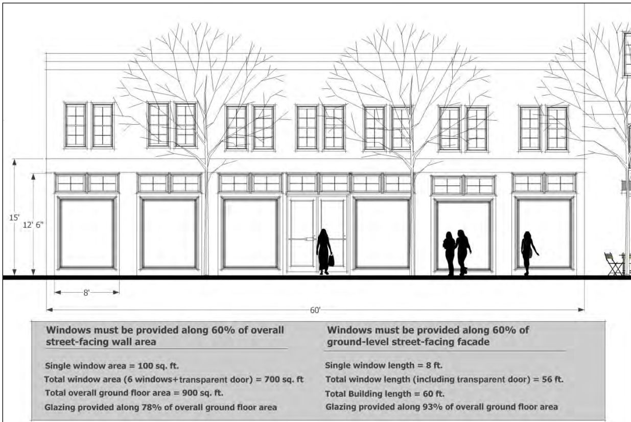
Figure 35 Illustration of percent transparency requirement
