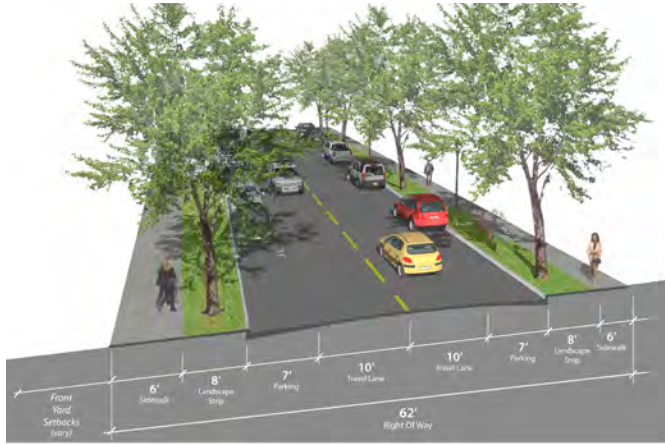
Figure 10: Typical Local Street Cross-Section
