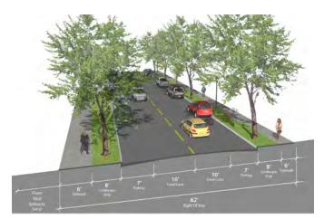
Figure 10: Typical Local Street Cross-Section
