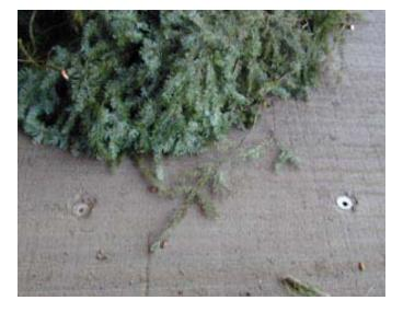
Air keeps the material from smelling sour. Air lines are inset in floor under material controlled to provide optimum amount of oxygen and cooling air.
