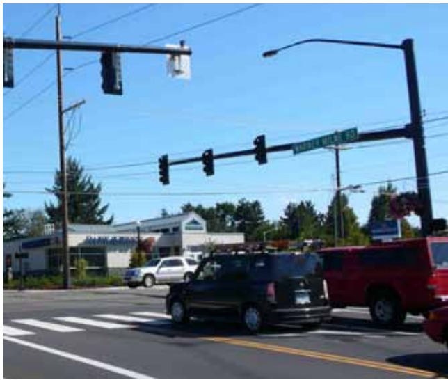
ORNAMENTAL SIGNAL POLES AND MAST ARM EXAMPLE
