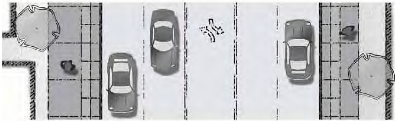
Figure 4: Landscape Easements. In most of the STA and Urban segments, the existing sidewalk corridor is less than 12-feet, making it too narrow to comfortably accommodate street trees with landscaped tree wells. (Note: A 12-foot sidewalk corridor with a furnishing zone allows pedestrians walking in opposite directions to pass comfortably. The recommendation is for 12-foot sidewalk corridors where possible.) Acquiring landscape easements in the front setbacks of the properties along the highway might be an opportunity to increase the ‘garden center’ qualities of the highway.
