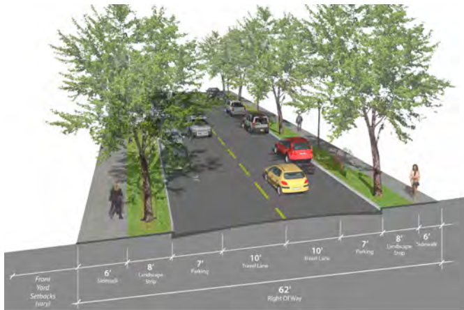
Figure 10: Typical Local Street Cross-Section
