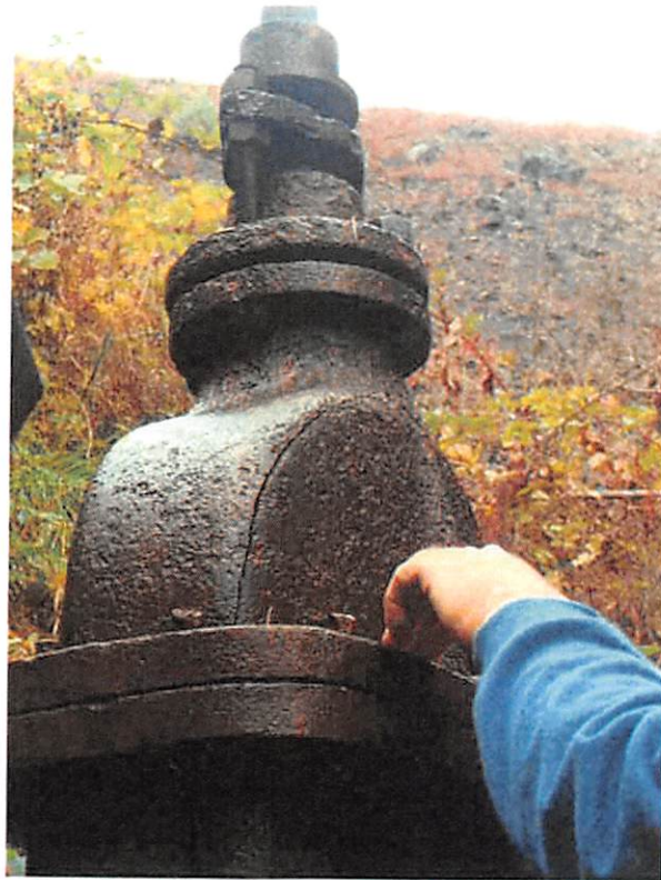
Crack in housing of upper most intermediate valve
